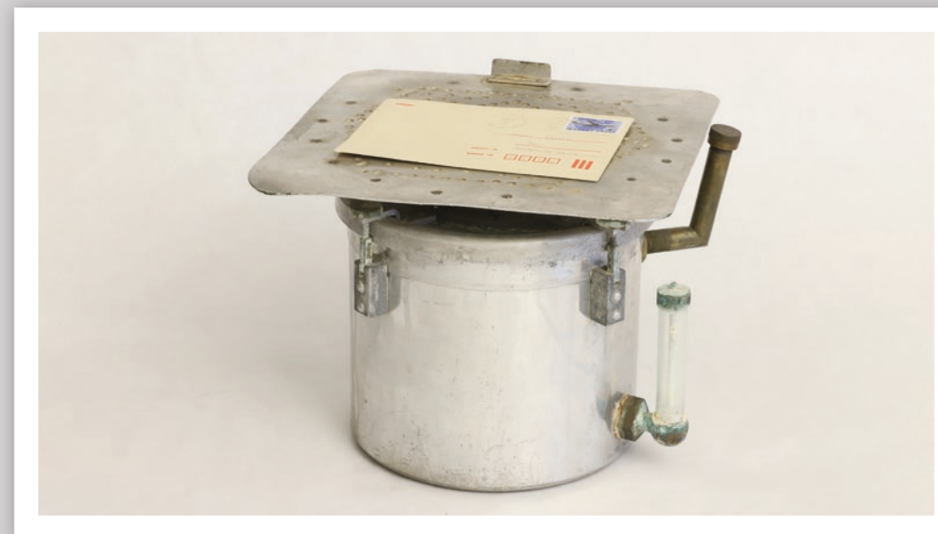
A letter opener, a device used for the opening of letters with steam (ÁBTL); photograph: Mihály Várai
